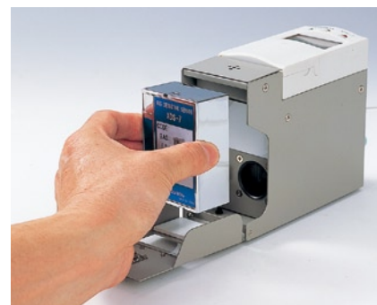
Remove the sensor unit and insert the new sensor unit. Close the sensor cover.
